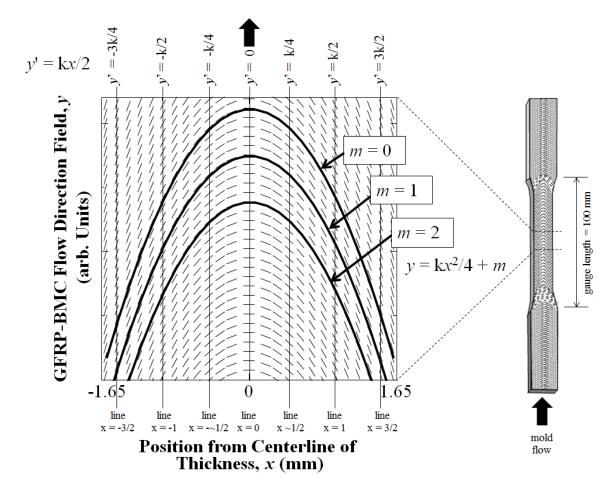
**Figure 2:** *GFRP-BMC* mold flow through dogbone specimen is represented as a flow direction field with slopes, y' = kx/2 (short lines) and its direct integration curves,  $y = kx^2/4 + m$ , where m is a constant, whose solution is a family of parabolas along specimen length. Note: small lines are not fibers.
